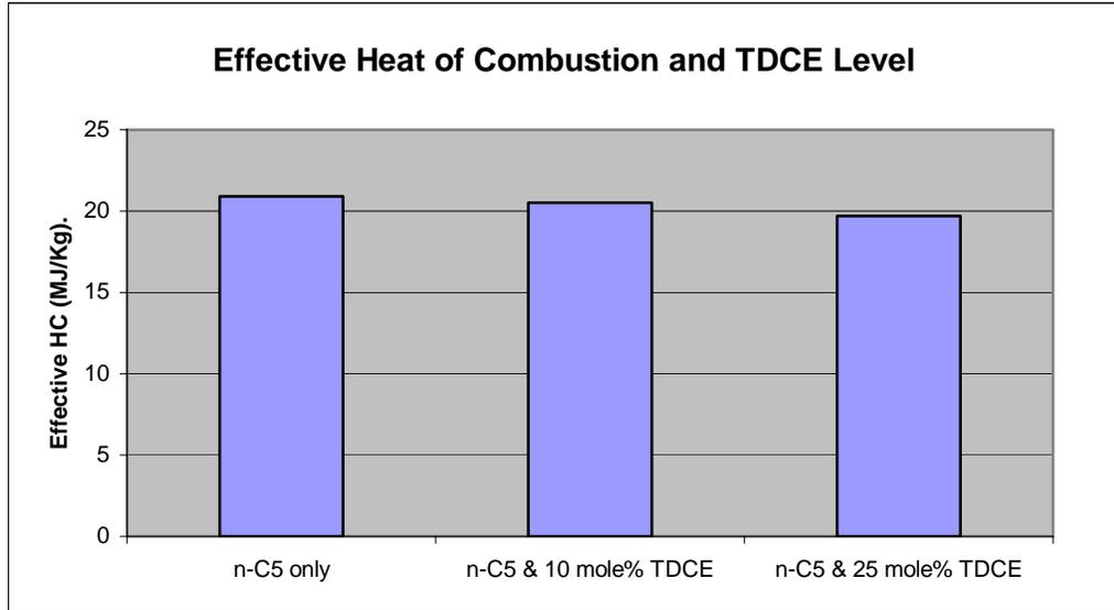
**Figure 4.** Effect of TDCE level on Heat Combustion of n-C5/TDCE Foams
