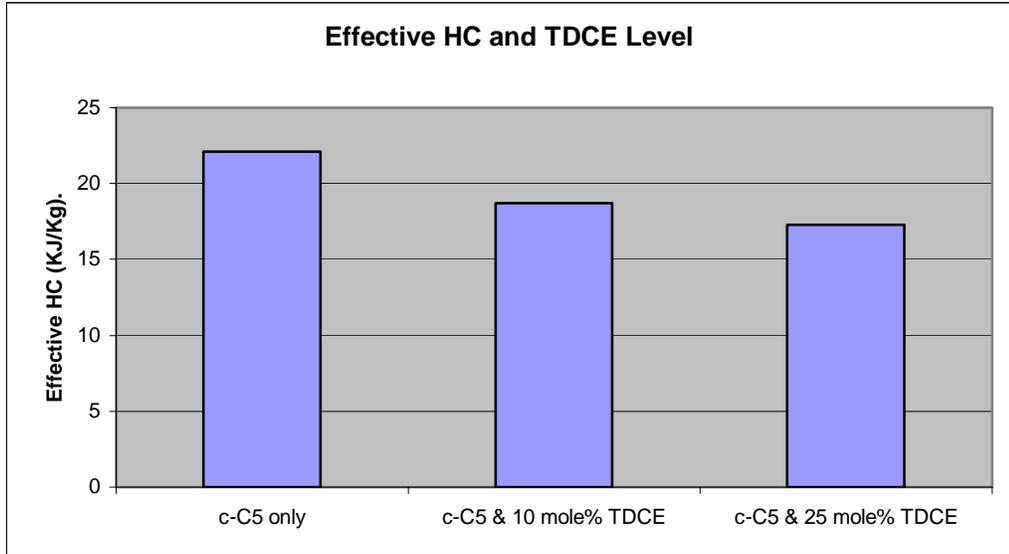
**Figure 16.** Effect of TDCE level on Heat Combustion of c-C5/TDCE Foams
