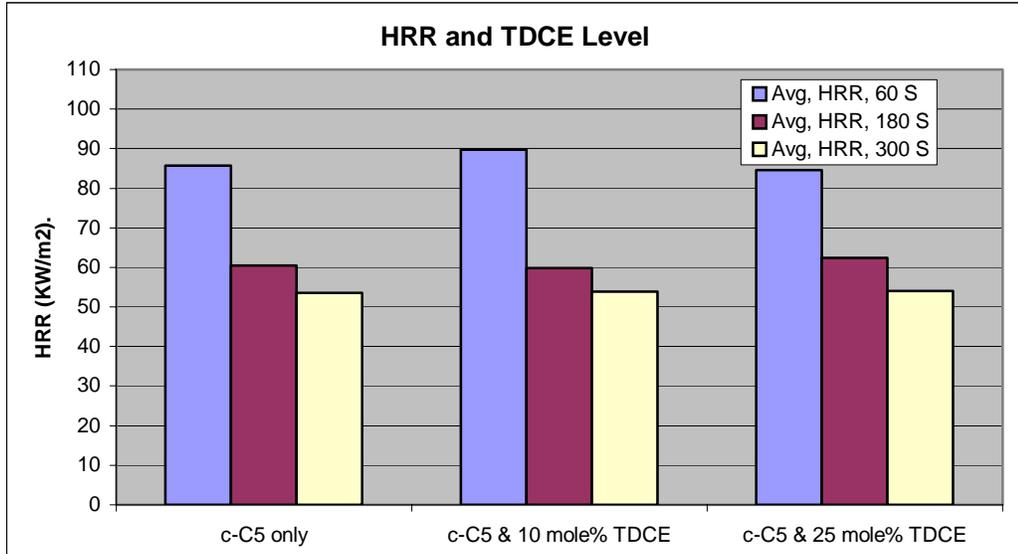
**Figure 14.** Effect of TDCE level on Heat Release Rate of c-C5/TDCE Foams
