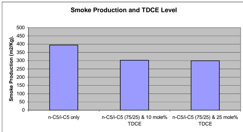
**Figure 11.** Effect of TDCE level on Smoke Production of n-C5/i-C5/TDCE Foams
