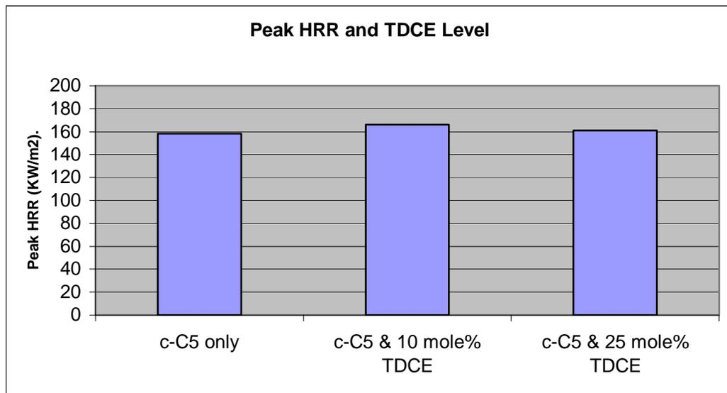
**Figure 13.** Effect of TDCE level on Peak Heat Release Rate of c-C5/TDCE Foams
