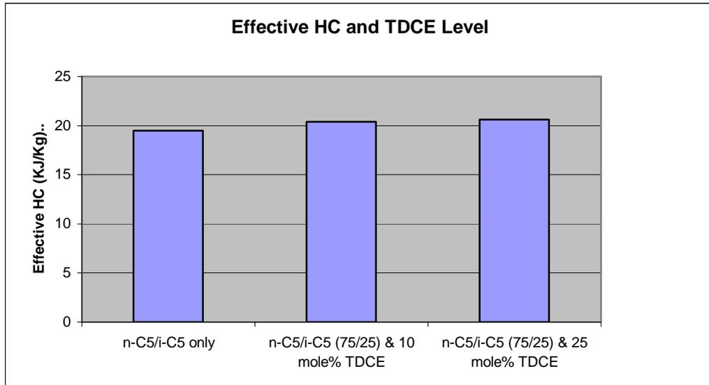
**Figure 12.** Effect of TDCE level on Heat Combustion of n-C5/i-C5/TDCE Foams
