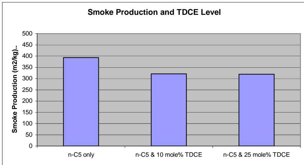
*Figure 3.* Effect of TDCE level on Smoke Production of n-C5/TDCE Foams
