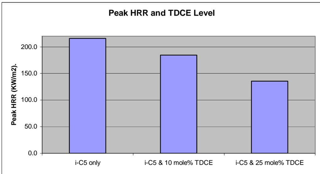
**Figure 5.** Effect of TDCE level on Peak Heat Release Rate of i-C5/TDCE Foams
