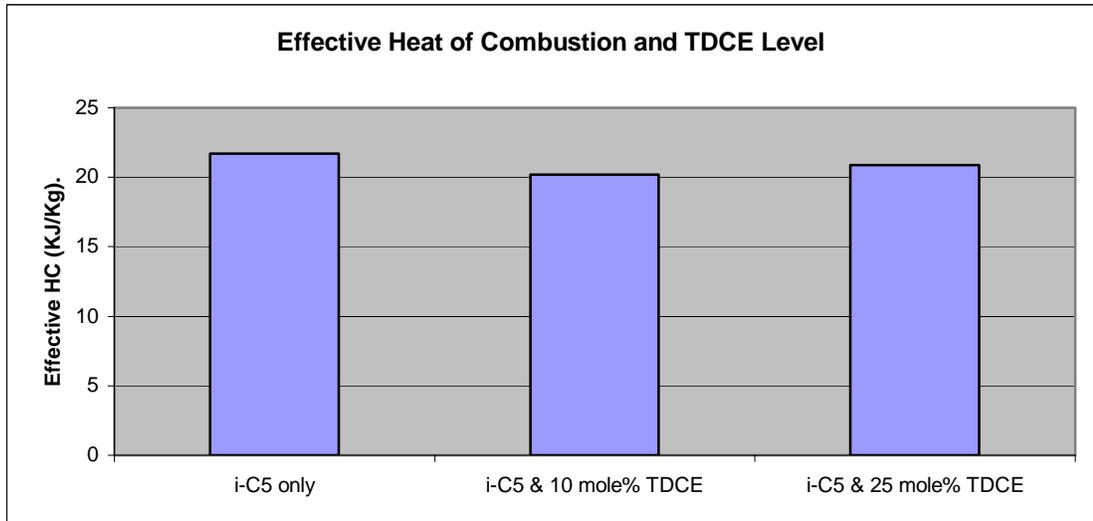
**Figure 8.** Effect of TDCE level on Heat Combustion of i-C5/TDCE Foams
