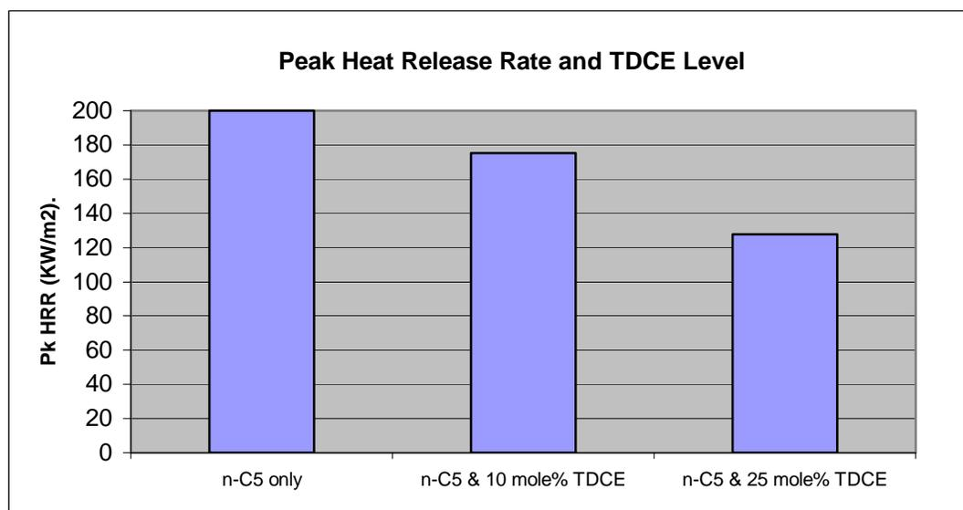
Figure 1. Effect of TDCE level on Peak Heat Release Rate of n-C<sub>5</sub>/TDCE Foams
