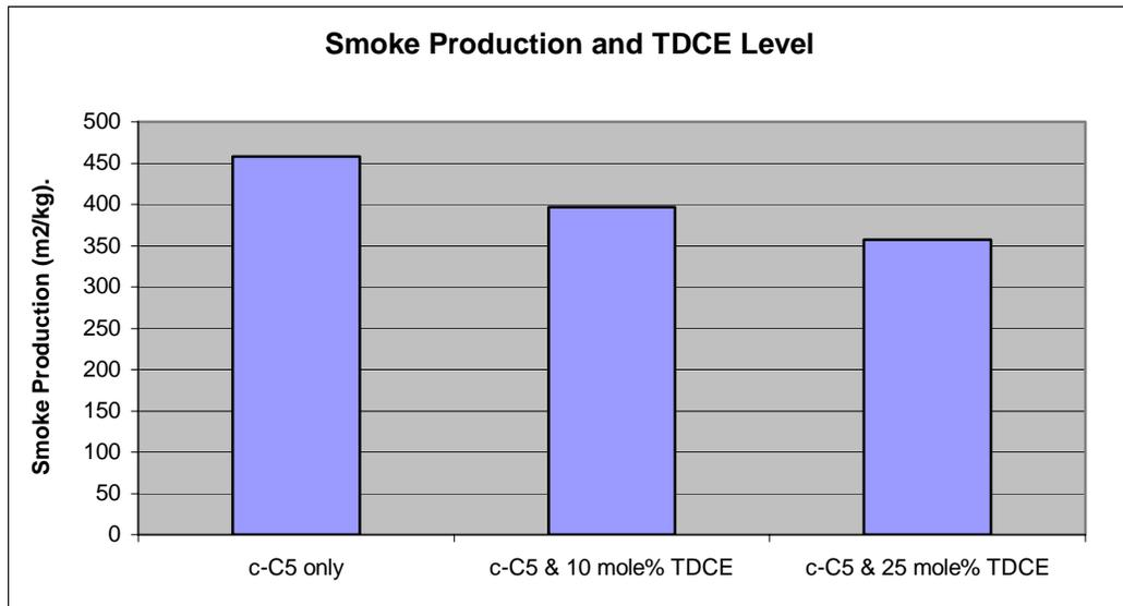
**Figure 15.** Effect of TDCE level on Smoke Production of c-C5/TDCE Foams
