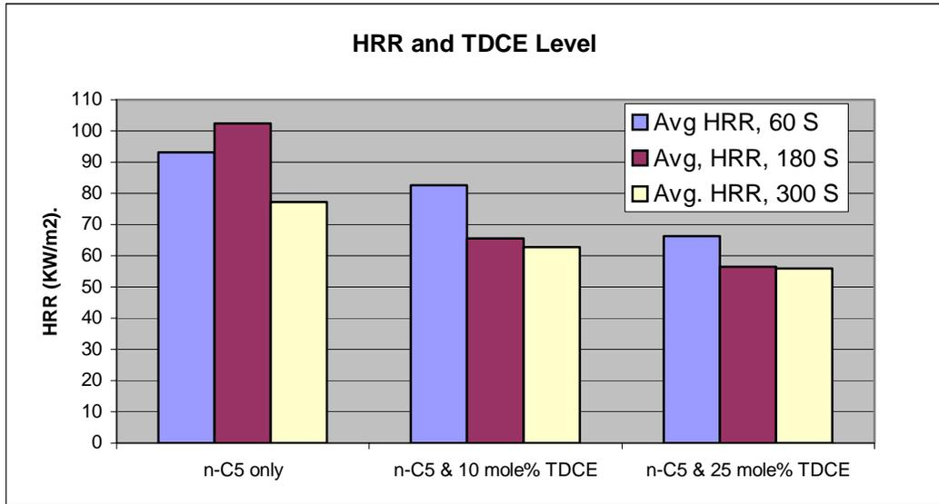
*Figure 2.* Effect of TDCE level on Heat Release Rate of n-C5/TDCE Foams
