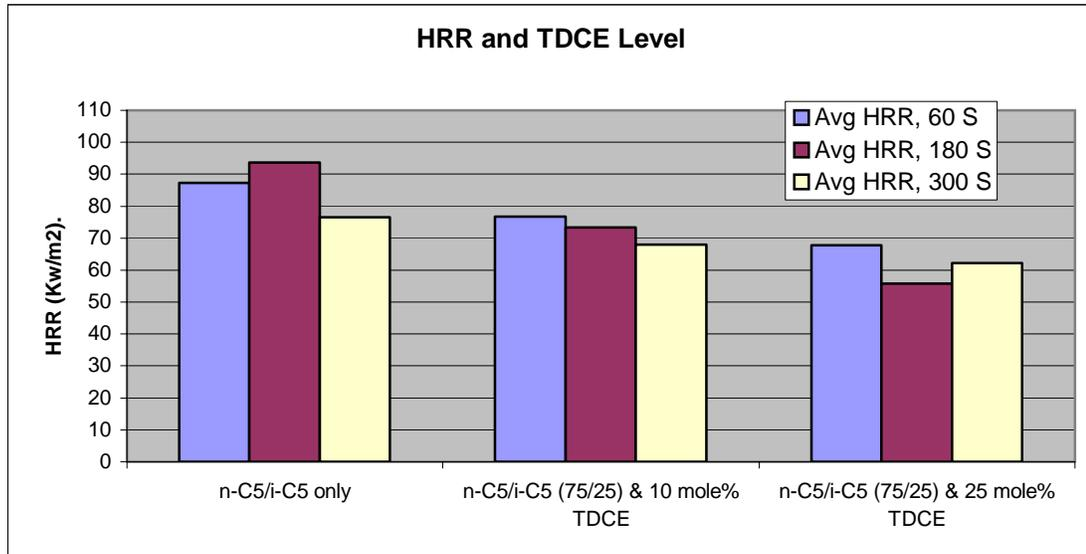
**Figure 10.** Effect of TDCE level on Heat Release Rate of n-C5/i-C5/TDCE Foams
