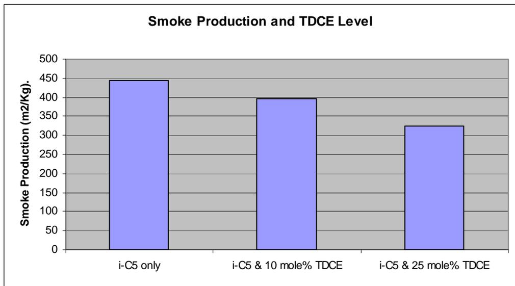
**Figure 7.** Effect of TDCE level on Smoke Production of i-C5/TDCE Foams
