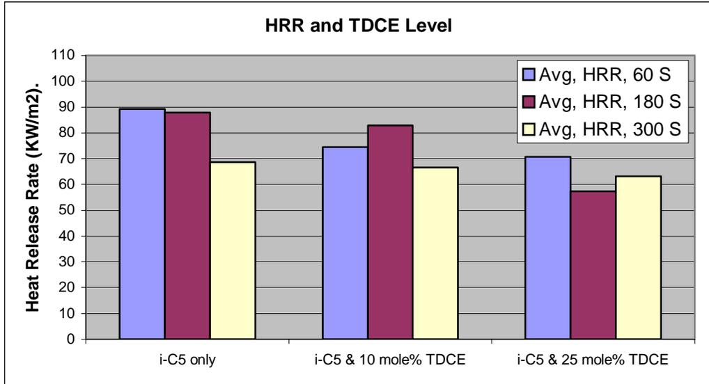
**Figure 6.** Effect of TDCE level on Heat Release Rate of i-C5/TDCE Foams
