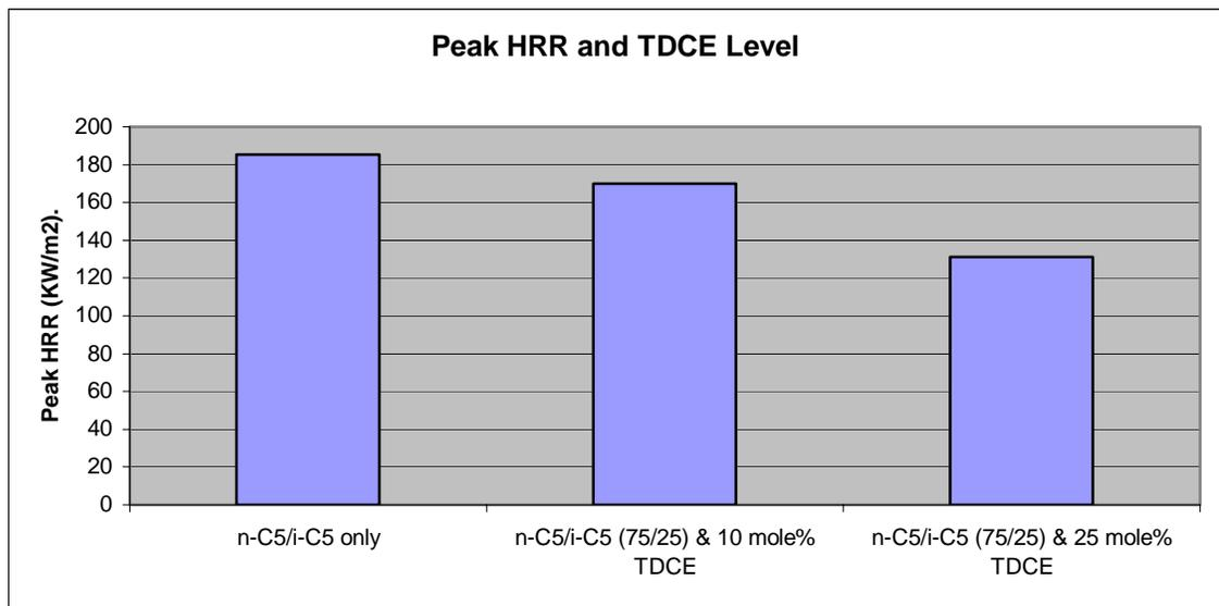
**Figure 9.** Effect of TDCE level on Peak Heat Release Rate of n-C5/i-C5/TDCE Foams
