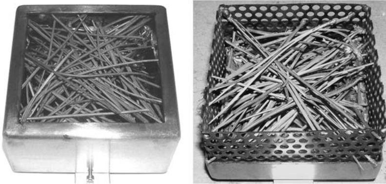
Figure 2. Standard holder (left) and porous holder (right) with samples of *Pinus pinaster* needles immediately before a test.
