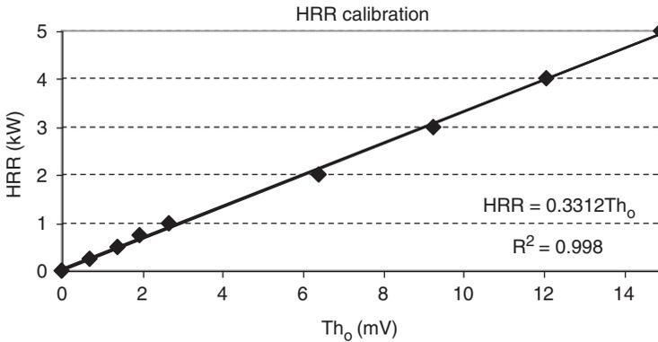
Figure 3. HRR calibration line for heat flux of  $50 \text{ kW/m}^2$ .  $Th_0$  is the change in thermopile output relative to the baseline generated at a heat flux of  $50 \text{ kW/m}^2$ .
