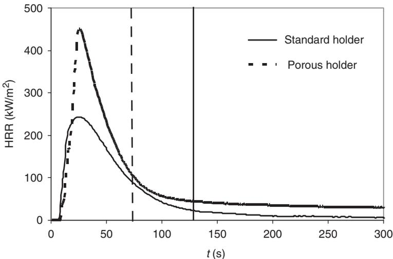
Figure 4. Comparison of HRR curves obtained for porous and standard holders in series of tests with *Pinus pinaster* (vertical lines indicate flameout).
