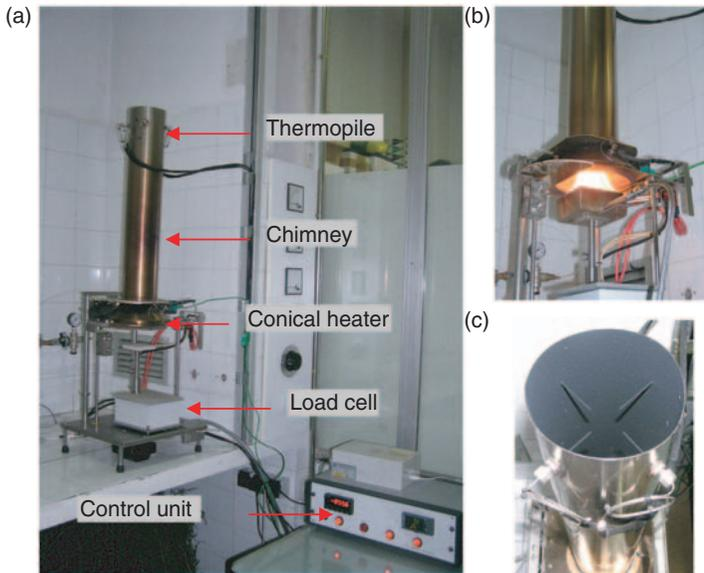
*Figure 1. (a) General view of the experimental device, (b) detail of methane burner used to calibrate the thermopile, (c) detail of the thermopile.*
