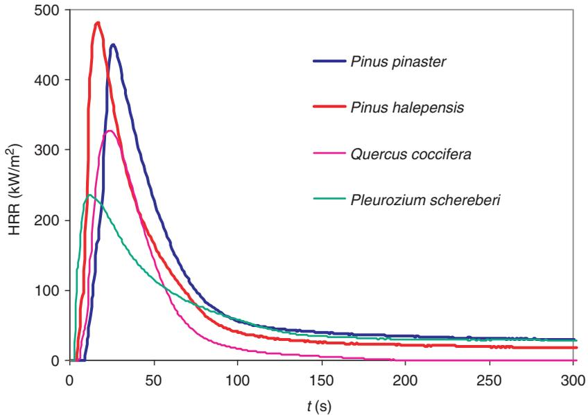
Figure 5. HRR curves for third series tests with a porous holder ( $n = 12$ ).
