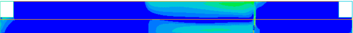
Figure 28 Velocity contours at a section through the centre of the tunnel at 5 minutes
