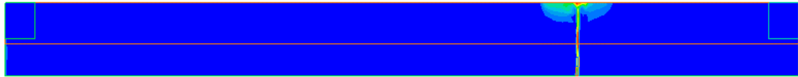
Figure 20 Velocity contours at a section through the centre of the tunnel at 1 minute
