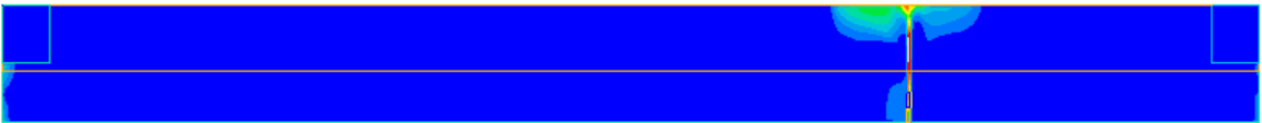
Figure 14 Velocity contours at a section through the centre of the tunnel at 1 minute
