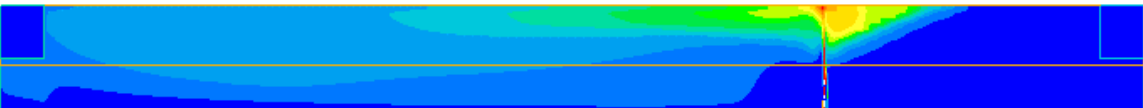
Figure 29 Temperature contours at a section through the centre of the tunnel at 10 minutes
