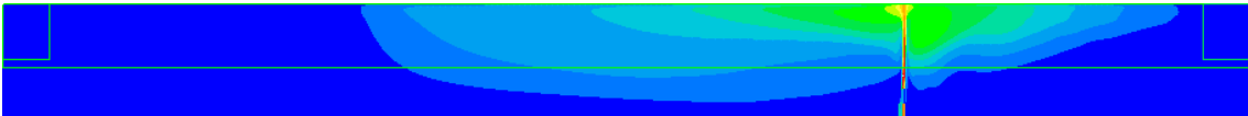
Figure 45 Temperature contours at a section through the centre of the tunnel at 5 minutes
