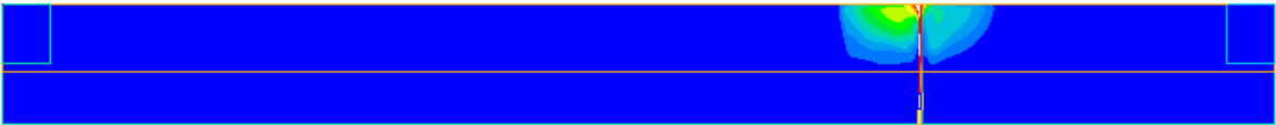
Figure 13 Temperature contours at a section through the centre of the tunnel at 1 minute
