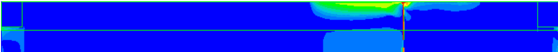
Figure 56 Velocity contours at a section through the centre of the tunnel at 1 minute
