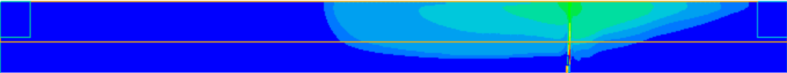
Figure 27 Temperature contours at a section through the centre of the tunnel at 5 minutes
