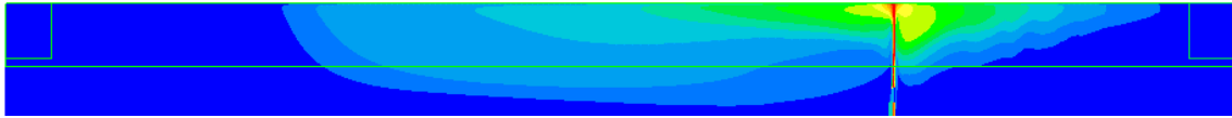
Figure 51 Temperature contours at a section through the centre of the tunnel at 5 minutes
