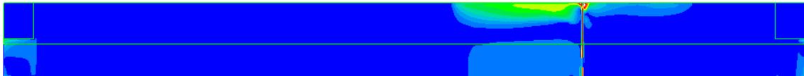
Figure 50 Velocity contours at a section through the centre of the tunnel at 1 minute
