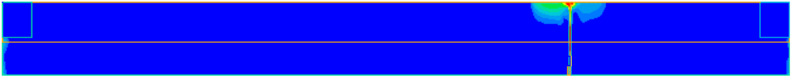
Figure 32 Velocity contours at a section through the centre of the tunnel at 1 minute
