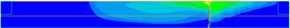
Figure 39 Temperature contours at a section through the centre of the tunnel at 5 minutes
