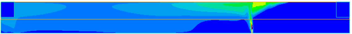
Figure 41 Temperature contours at a section through the centre of the tunnel at 10 minutes
