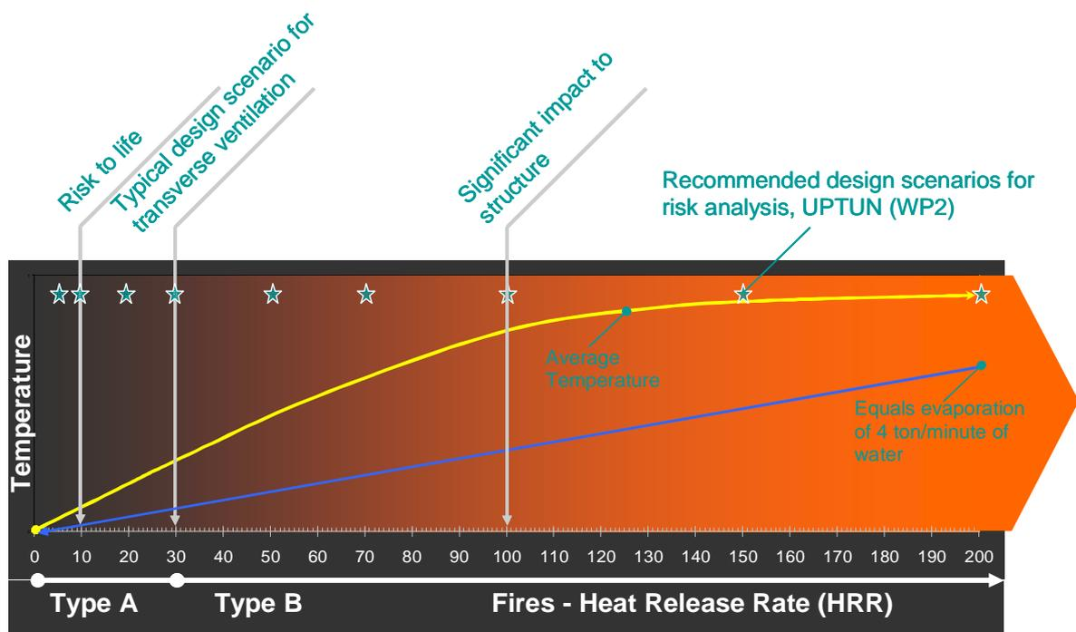
Figure 1. shows the Type A) fires where mitigation action should be provided, while Type B) often represents fires out of control and may provide significant heat exposure to the structure. For risk analysis several scenarios are recommended, her shown by stars<sup>15</sup>.
