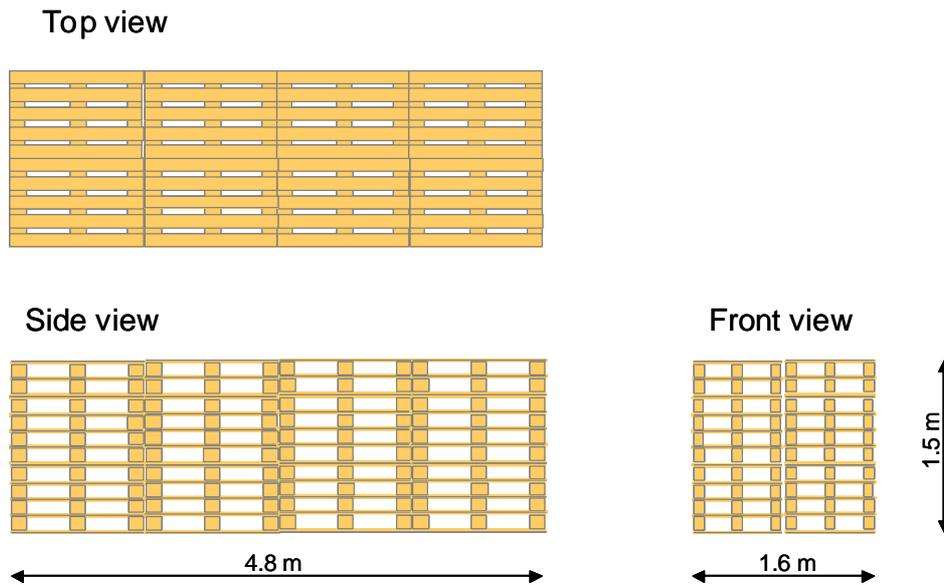
Figure 3. The drawing shows the solid fuel test commodity
