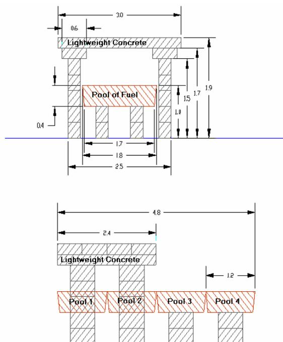
Figure 2 The drawing shows the experimental setup of sheltered pool fires. The fuel was diesel and the ventilation direction was from left to right (all dimensions in meters)
