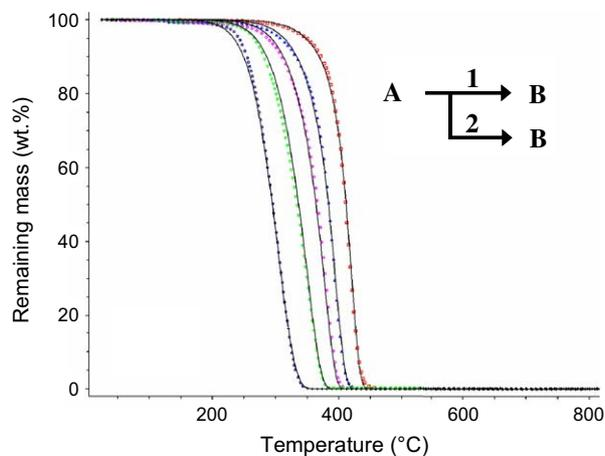
Fig. 6. Experimental (dots) and simulated (line) TG curves of pure polystyrene (N<sub>2</sub> flow).
