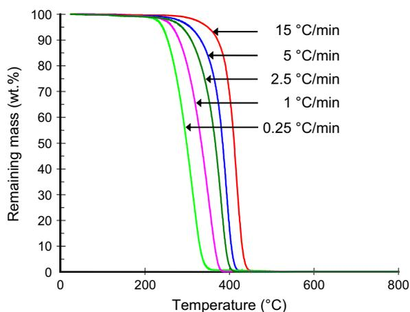
Fig. 4. TG curves of pure polystyrene versus heating rate (N<sub>2</sub> flow).
