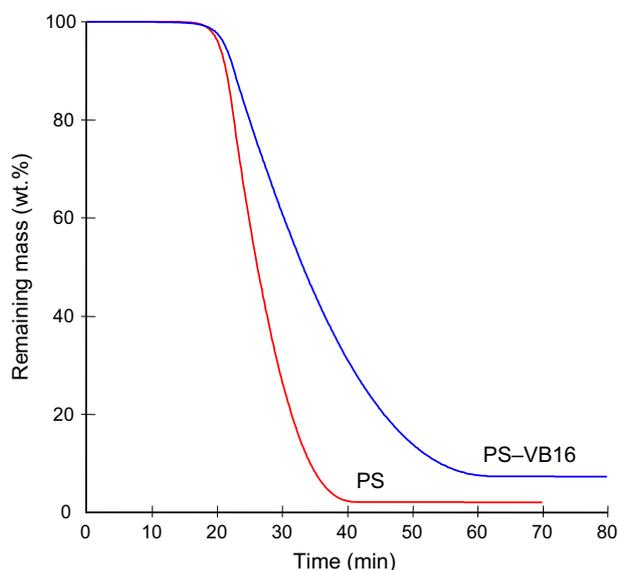
Fig. 18. Simulated curves of the thermo-oxidative degradation of PS and PS–VB16 in isothermal conditions at 350 °C after a ramp of 20 °C/min.
