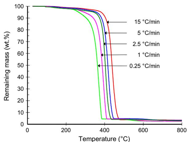
Fig. 13. TG curves of PS–VB16 versus heating rate (N<sub>2</sub> flow).
