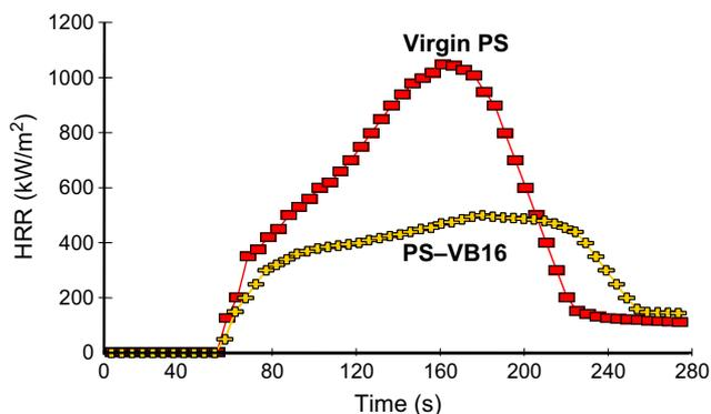
Fig. 1. Heat release rate (HRR) curves versus time of virgin PS and PS–VB16 nanocomposites (external heat flux = 35 kW/m<sup>2</sup>).
