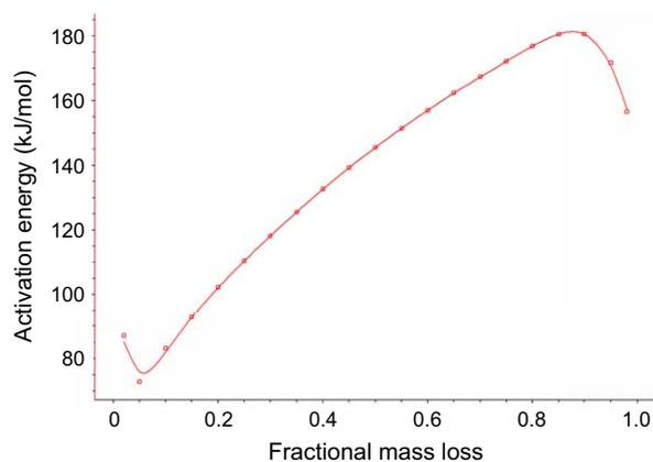
Fig. 5. Activation energies of pure PS versus fractional mass loss determined using the Friedman analysis (N<sub>2</sub> flow).
