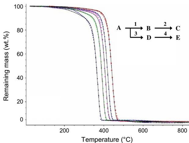
Fig. 16. Experimental (dots) and simulated (line) TG curves of PS–VB16 ( $N_2$  flow).
