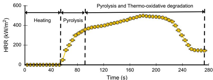
Fig. 19. Assignment of different sections of the HRR curve of PS–VB16 versus time (external heat flux = 35 kW/m<sup>2</sup>).
