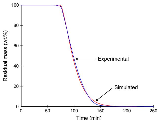
Fig. 7. Experimental and simulated degradation curves of pure PS at 350 °C for 250 min ( $N_2$  flow).
