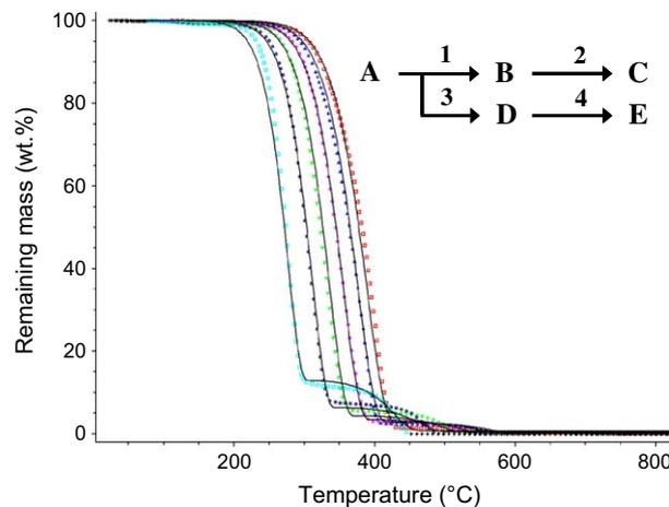
Fig. 11. Experimental (dots) and simulated (line) TG curves of pure polystyrene (air flow).
