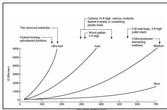
**Figure 5 - Standard Fire Growth Rate Curves. (with some examples of fire test fuels)<sup>51</sup>**
