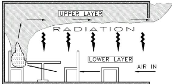
Figure 2 – Pre-flashover conditions in a compartment fire.
