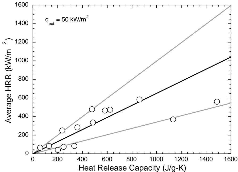
FIGURE 3. AVERAGE HRR IN FLAMING COMBUSTION VERSUS HEAT RELEASE CAPACITY OF 14 COMMERCIAL PLASTICS.
