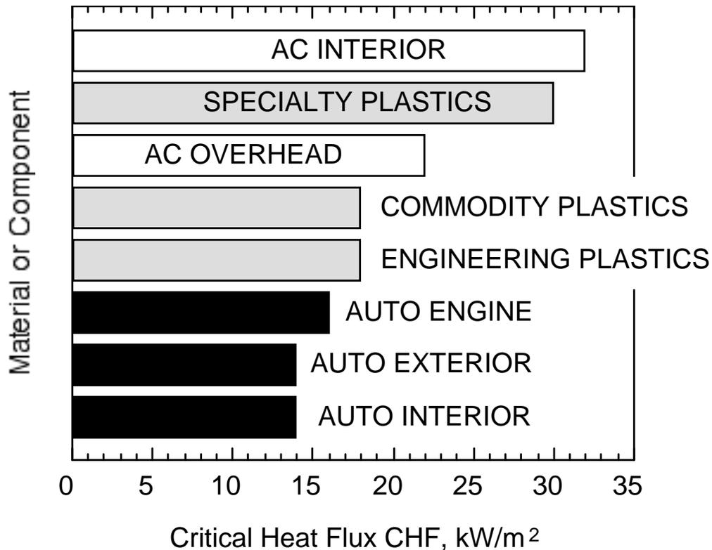
FIGURE 8. IGNITION RESISTANCE OF MATERIALS AND COMPONENTS RANKED BY CRITICAL HEAT FLUX.
