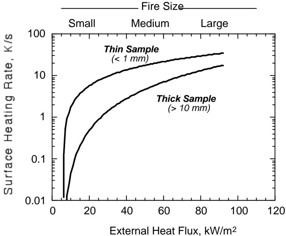
FIGURE 1. SURFACE HEATING RATES OF THIN AND THICK PLASTIC SAMPLE FOR VARIOUS FIRE SIZES.
