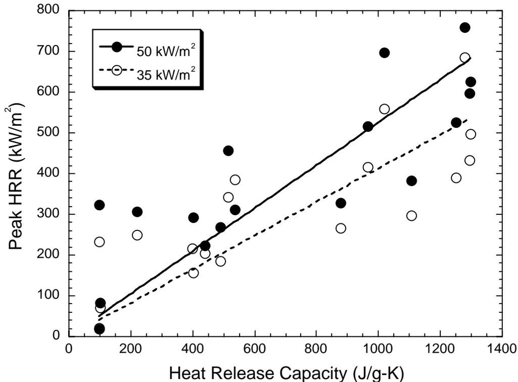
FIGURE 6. PEAK HEAT RELEASE RATE FROM THE CONE CALORIMETER AT 35 AND 50 kW/m<sup>2</sup> VERSUS THE HEAT RELEASE CAPACITY FROM THE MICROSCALE COMBUSTION CALORIMETER.
