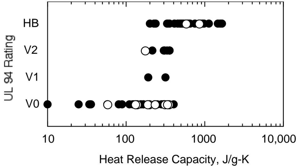
FIGURE 4. FLAMMABILITY RATING OF COMMERCIAL PLASTICS IN UL 94 TEST VERSUS HEAT RELEASE CAPACITY (OPEN CIRCLES ARE HALOGEN CONTAINING PLASTICS).
