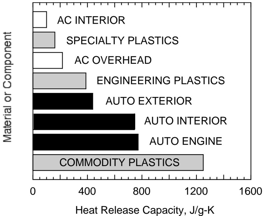
FIGURE 7. FLAMMABILITY OF PLASTIC COMPONENTS AND MATERIALS BY APPLICATION RANKED BY HEAT RELEASE CAPACITY.
