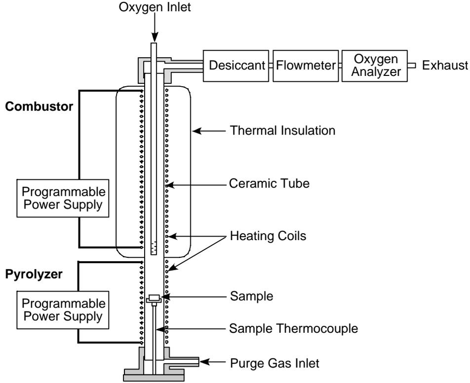
FIGURE 2. SCHEMATIC DRAWING OF PCFC SHOWING PYROLYZER, COMBUSTOR, GAS CONDITIONING, AND MEASURING COMPONENTS.
