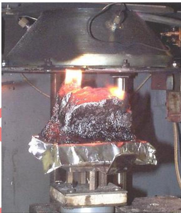
*On line analysis of the degradation product with the IRTF*
